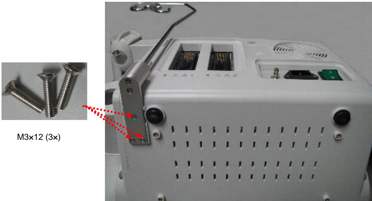
Figure 4-1 Assembling Cable Holder to Main Unit
